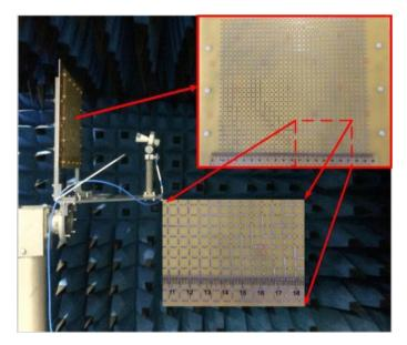
Figure 1: 32x32 element prototype offset reflectarray under test [2].
